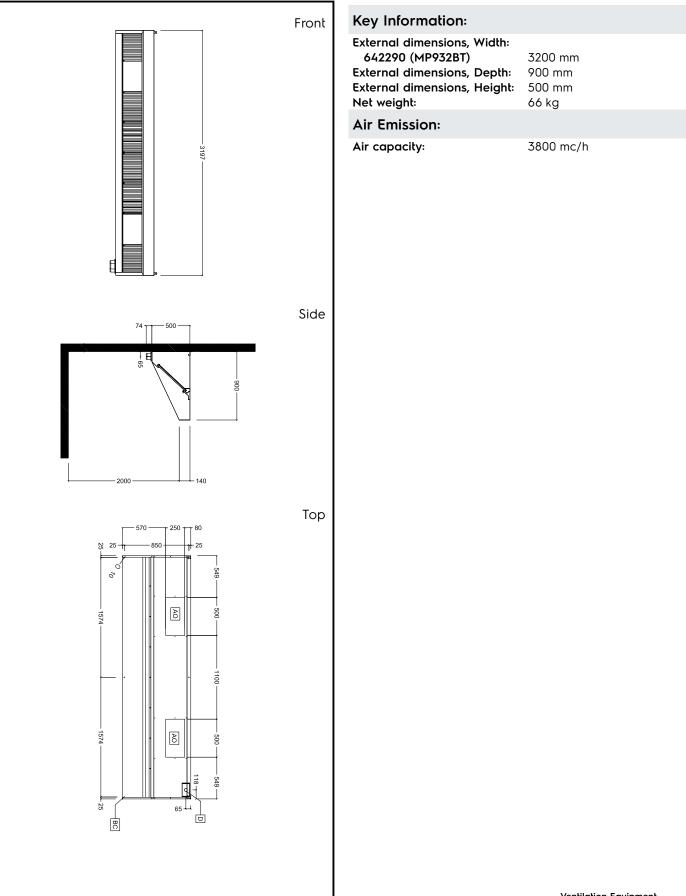
Ventilation Equipment 430 S/S Wall Hood+Filters 3200X900mm
